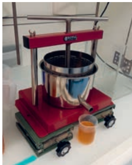
Photo 2: Fruit press tested to dewater conditioned faecal sludge.
