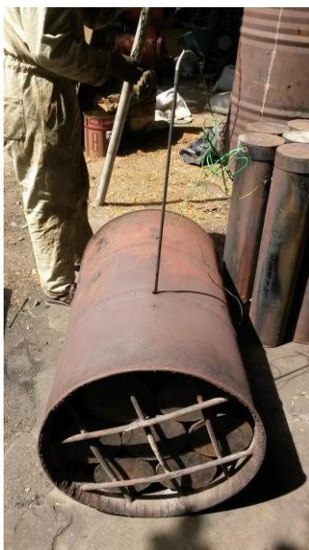
Figure 72: Insertion of the thermocouple through the barrel wall
