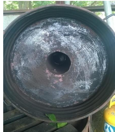
Figure 65: Left: produced char emptied on a plastic or cardboard sheet (T4.7). Right: Clean chimney after removing the soot with the wire brush (T4.9)
