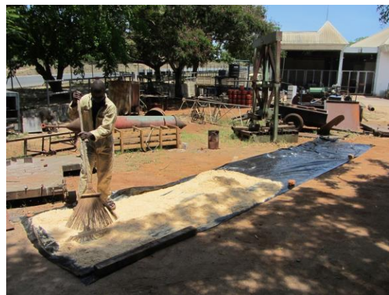
Figure 46: Sun pre-drying sawdust.
