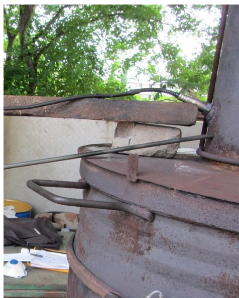
Figure 74: Connecting the Lambda sensor and the thermocouple to the chimney.
