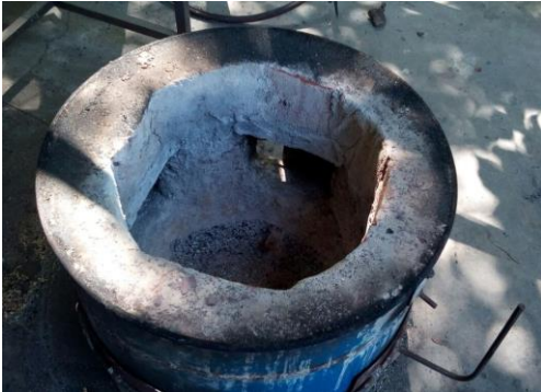
Figure 14: Insulation of the furnace made with bricks and mortar.
