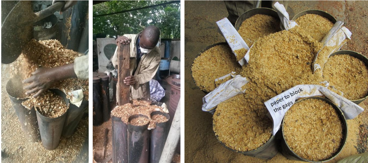
Figure 47: Filling, compressing the feedstock in the tubes (T1.3)
