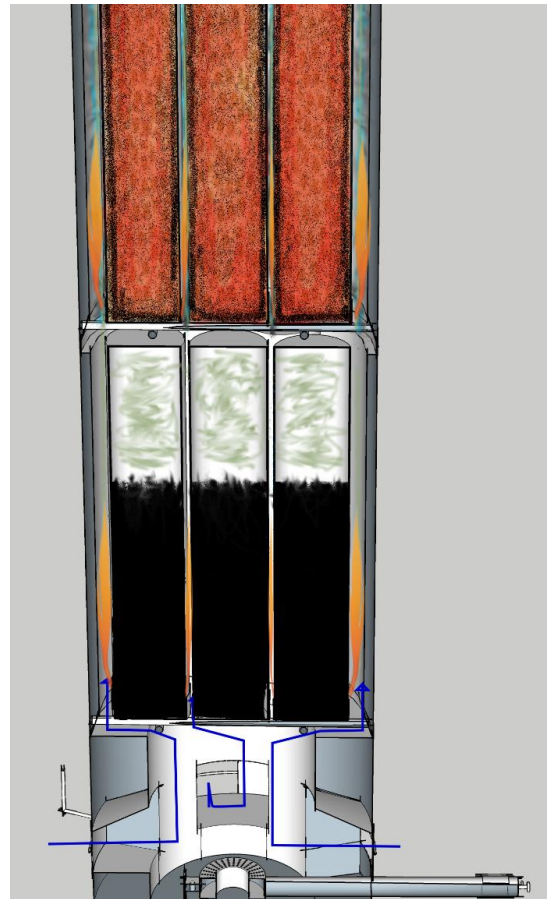
Figure 59: Schematic of the pyrolysis process. Lower barrel fully carbonized. Upper barrel: beginning of the pyrolysis process
