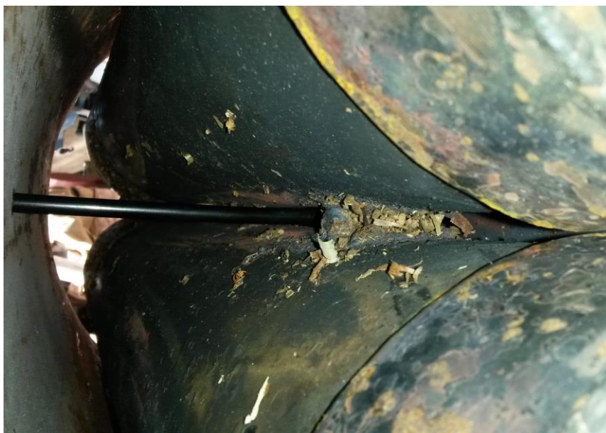
Figure 73: Thermocouple in the interior of the barrel.
