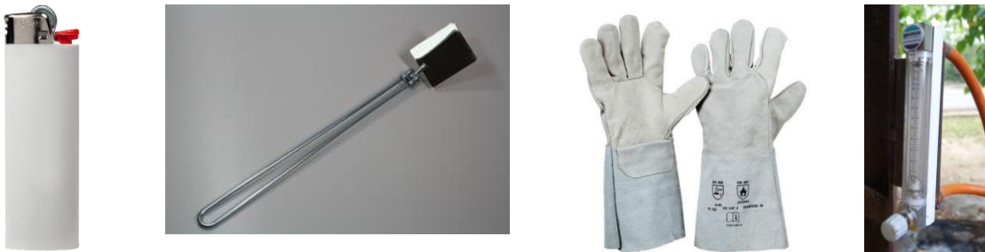
Figure 52: Left: lighter or matches. Middle1 : Mirror with handle. Middle 2: Thermoresistant gloves. Right: Rotameter. Model: Wagner, C 4 H 10 , 2-19l/min
