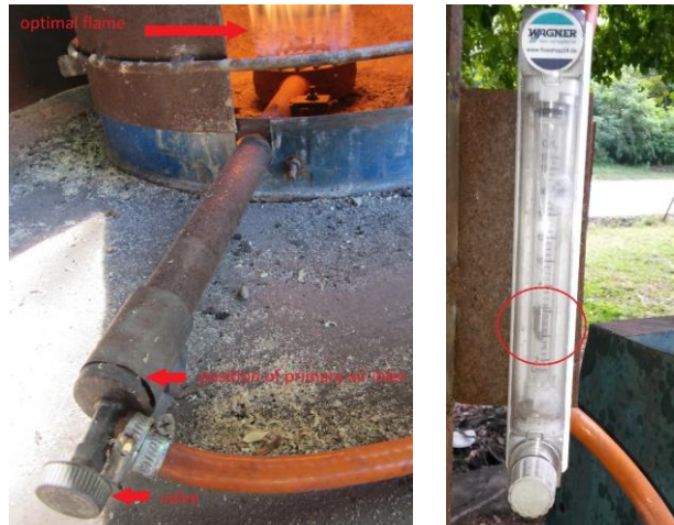
Figure 53: Valve of burner to adjust LPG flow (lower red arrow). Black cover to adjust primary air entering the burner (upper red arrow).
