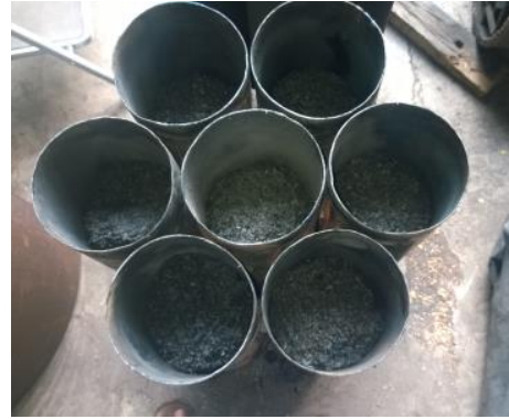
Figure 64: Volume loss of the feedstock after pyrolysis process.
