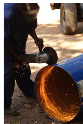
Figure 10: Cutting the barrel with a cutting disk.
