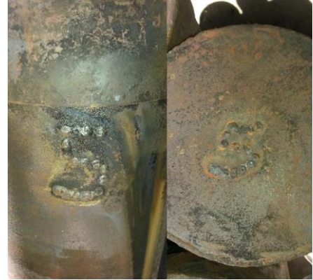
Figure 32: Numbering used to identify best fitting lids and tubes.
