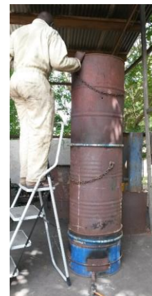
Figure 51: Locating upper barrel and chimney with ladder (T1.5 and T1.6)
