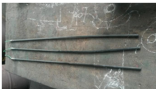
Figure 69: Overview of the thermocouples used.
