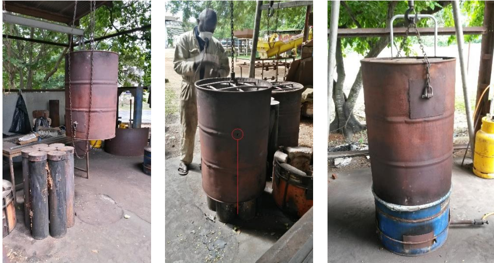
Figure 49: Assembling the reactor barrel: bringing the barrel and tubes together (T1.4)
