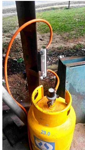
Figure 44: Left: gas cylinder and rotameter. Right: three barrel straps to fix the barrels.
