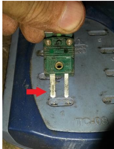
Figure 76: Connecting thermocouples to PicoLog hub (T2.3)
