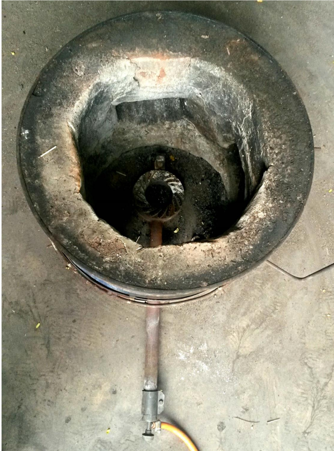
Figure 19: Top view of furnace
