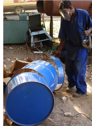
Figure 12: Barrel separated into three parts
