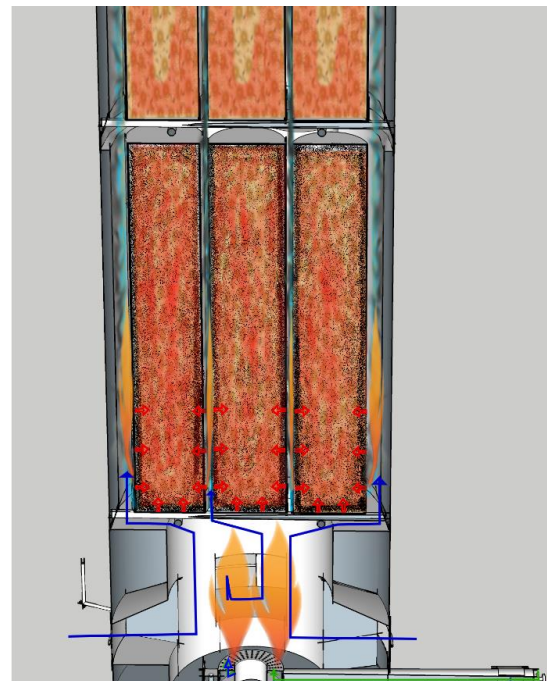
Figure 58: Schematic of the carbonization process in the lower barrel: heat distribution, combustion of the pyrolysis gases and supply of secondary air.
