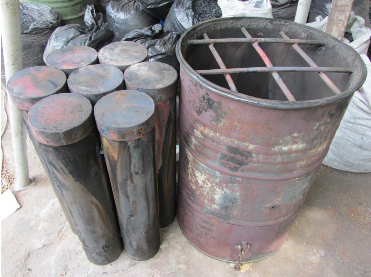
Figure 20: Overview of one oil barrel and its seven tubes.
