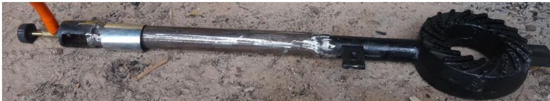
Figure 18: Photo of the burner, with welded extension
