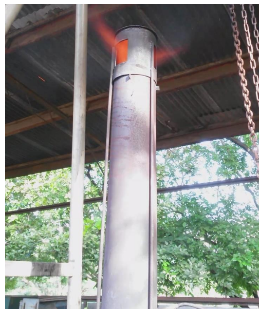
Figure 60: Strong pyrolysis in the upper barrel with flames coming out of the chimney.
