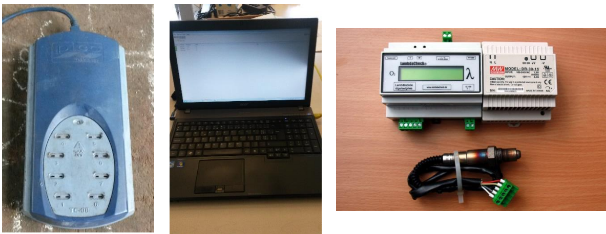
Figure 71: Left: PicoLog hub with USB-cable. Middle: Laptop with PicoLog software. Right: LambdaCheck unit (top) and the sensor (bottom) to measure the residual oxygen.
