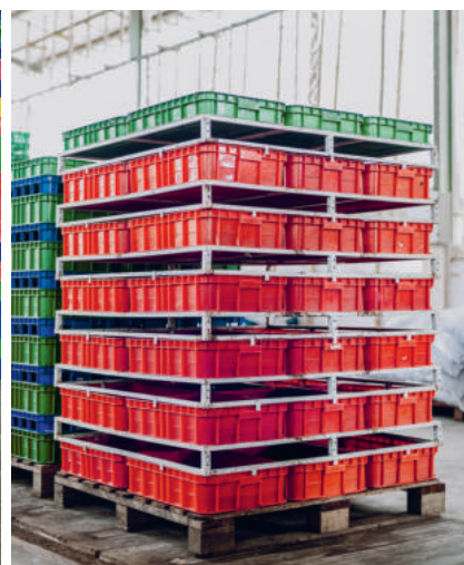
Figure 4–6: Stack of larveros with ventilation frames in-between levels
