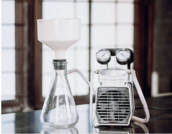
Step 1: Vacuum pump setup.
