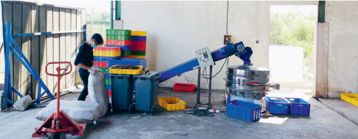
Step 1: Harvesting station with sieving system, collection bins and residue bags
