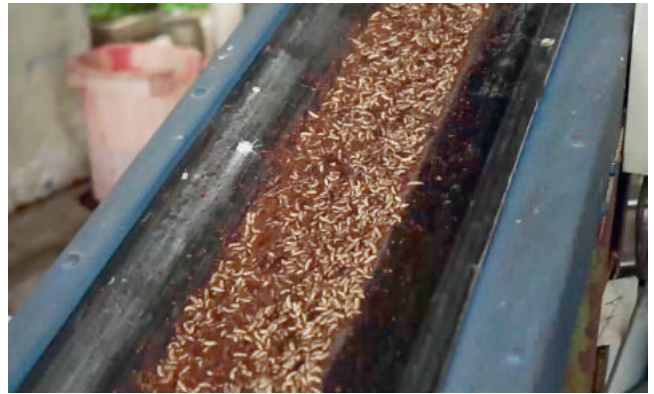
Step 7: Larvae and residue on transport belt before being separated into the different fractions
