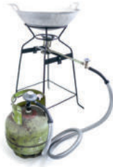
Wok pan setup Diameter pan: 30 cm Capacity: 3 kg/h
