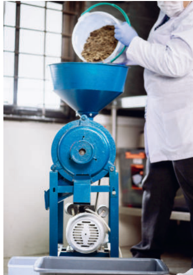
Step 2: Adding of press cake to the grinder.
