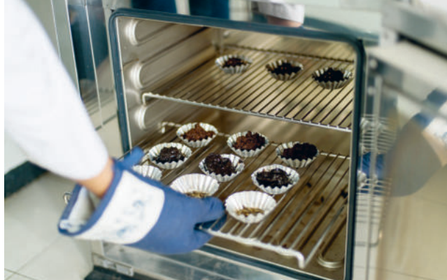
Triplet samples of substrate in, residue out and larvae out are placed in the TS oven
