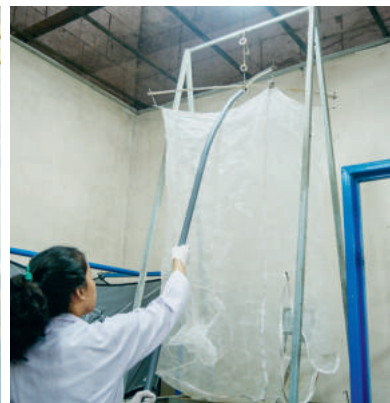
Step 2: Using the cage moving stick to hang love cage into mobile frame
