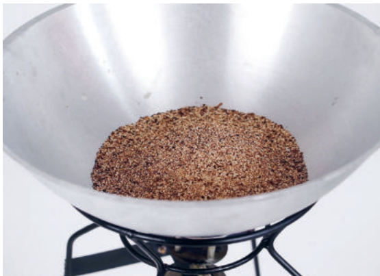
Step 1: Preheating 1 kg sand in a wok pan.
