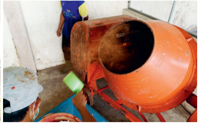
Step 6 + 7: Conditioning of substrate by adding dry material if water content is too high and adding water if water content is too low
