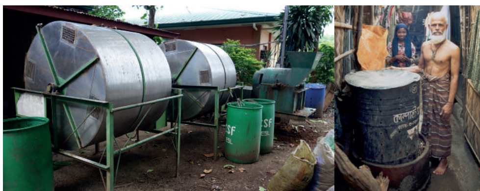
Figure 5: Small scale In-vessel composting drums (left) and Bin composting in India (right)
