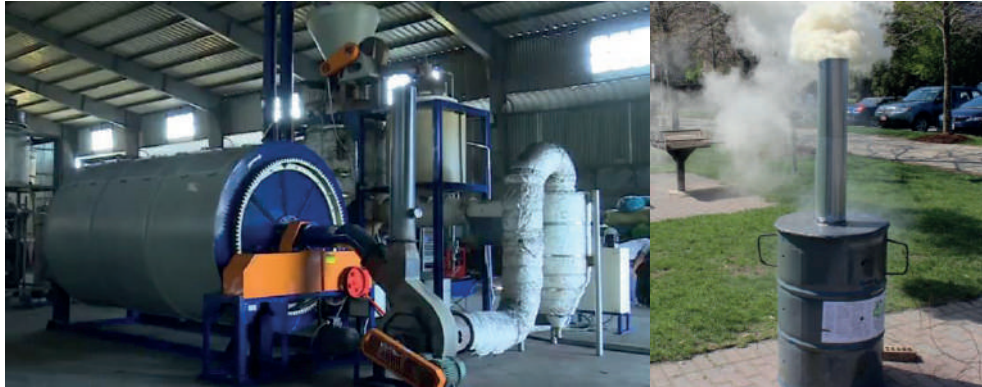
Figure 18: Continuous slow pyrolysis system, Vietnam (photo: Ökozentrum, Sofies) – (left) and ARTI style drum (photo: Dan Sweeney) (right)
