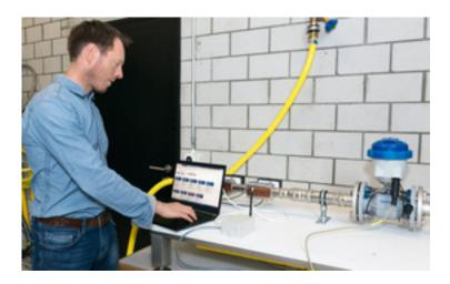
Dr. Frank Blumensaat (Urban Water Management department) uses ADAWIM for wireless measurement of the water flow in the test assembly. (Foto: Patrick Cipriani / ZHAW)
