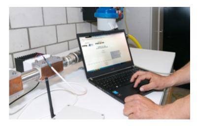
Wireless measurement of the flow in the test assembly. (Foto: Patrick Cipriani / ZHAW)
