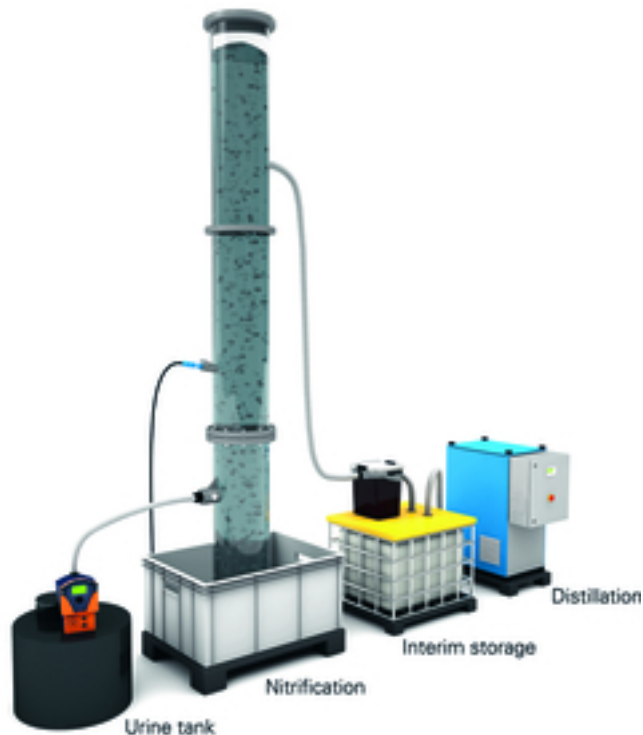
Fig. 2: The urine separation and treatment technology developed in the VUNA project is also being used in the Water Hub project. In a nitrification and distillation system, nutrients are recovered from source-separated urine to produce a fertilizer. (Photo: Eawag)
