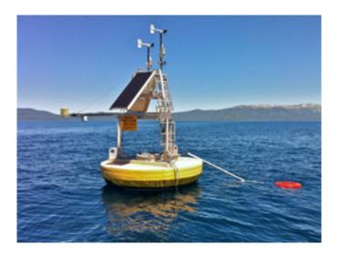
A combination of satellite data and ground measurements, such as from instrumented buoys like this one in Lake Tahoe on the California/Nevada border, were used to provide a comprehensive view of changing lake temperatures worldwide. The buoy measures the water temperature from above and below. *Credits: Limnotech*
