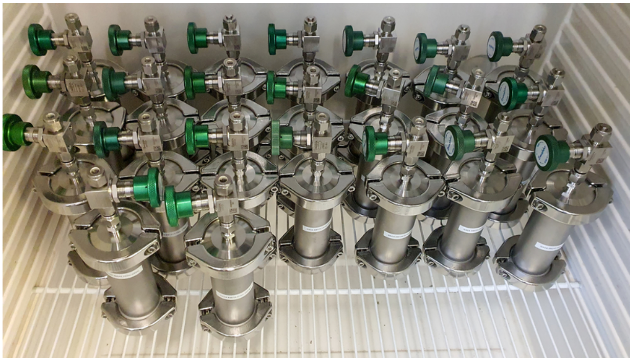
Sections from the sediment core ready for analysis of the pore space water using the portable mass spectrometer GE-MIMS (the “Mini-Ruedi”) developed by Eawag (Photo: Yama Tomonaga, Eawag, University of Basel).
