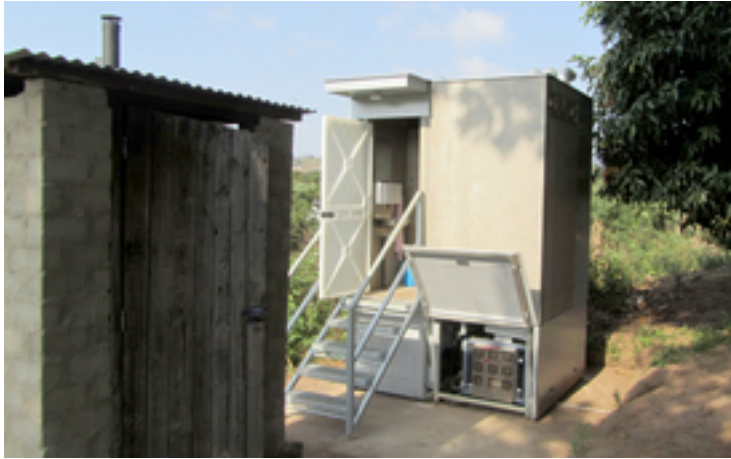
The Blue Diversion Autarky toilet in test on the outskirts of Durban, South Africa. The evaporation module is visible in the front right. (Michel Riechmann, Eawag)
