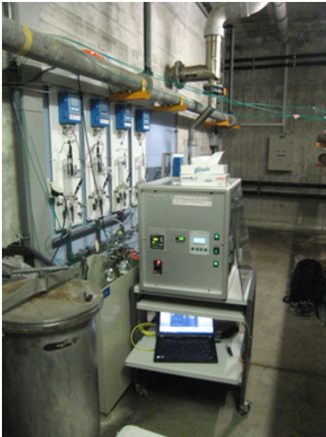
Fig. 2: Equipment used for continuous measurement of trichloramine at various points in the pool water circulation system. (Photo:
