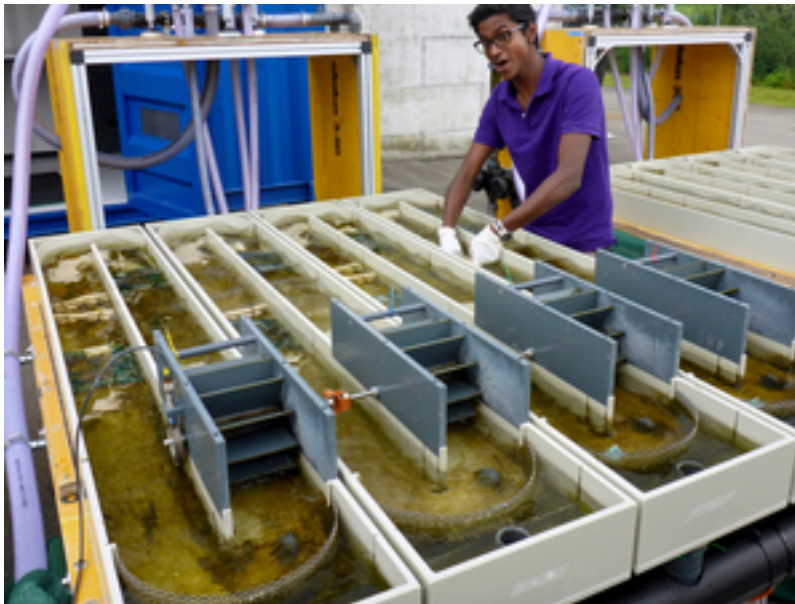
Fig. 4: A 16-channel flume system was used to study the effects of different constituents of wastewater. (Photo: Eawag)
