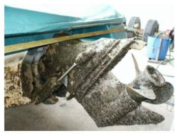
Virtually all of Switzerland's navigable waters are connected via overland boat movements – the thicker the lines, the more frequently the transport routes are used (left). Sterndrive encrusted with zebra mussels (right).
