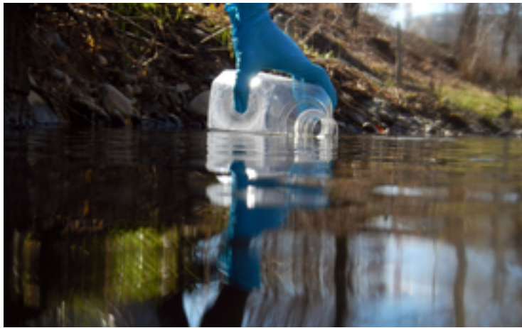
Taking a water sample for subsequent analysis of the environmental DNA (Photo: Eawag, Elvira Mächler)
