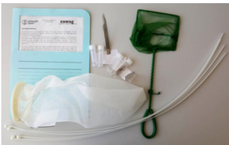
The sampling material with which the water supply managers involved in the project were equipped. Photo:
