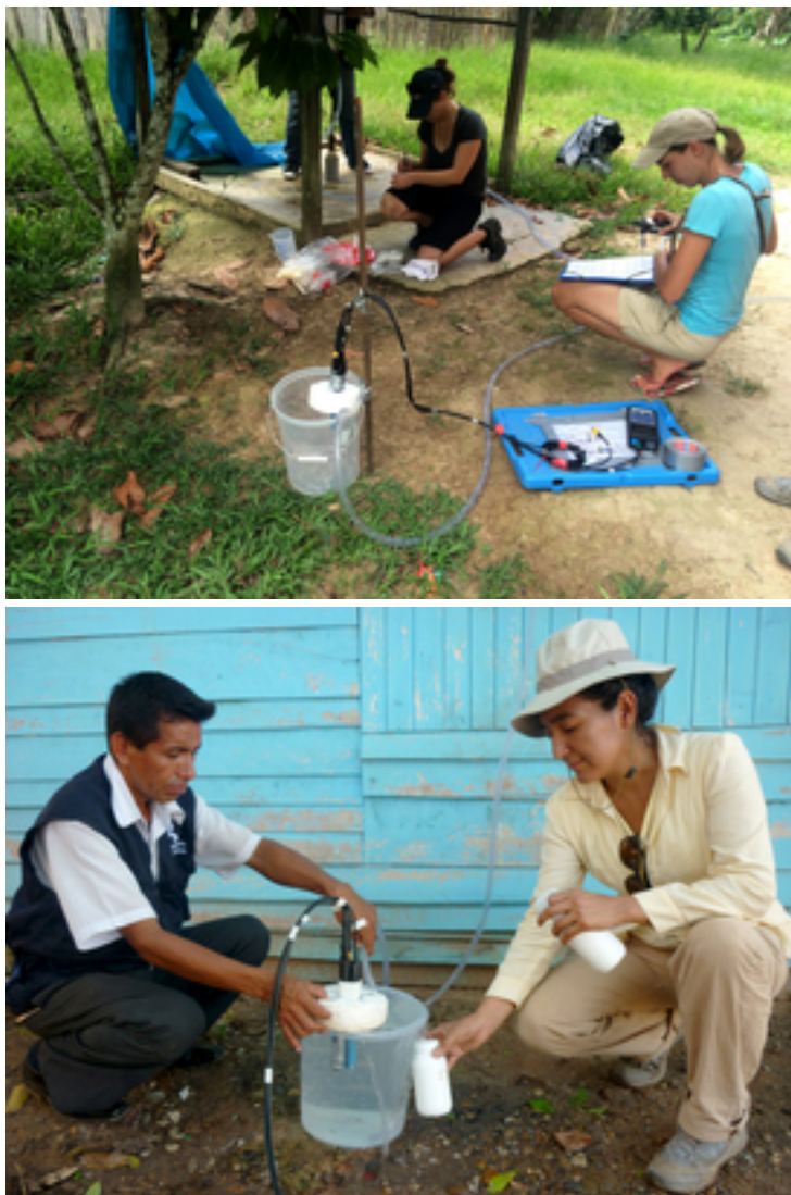
A typical groundwater well and scientists measuring geochemical parameters in Peru. (Photos: Caroline de Meyer, Eawag and Edward Carpio Deza, Universidad Nacional de Ingeniería, Lima).
