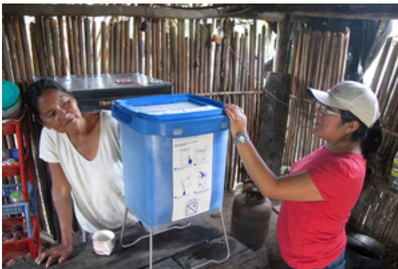
Prototype of the GDM household filter in a field test in Peru. With a membrane surface of 0.5 m 2 , the filter can supply up to 30 litres of drinking water a day – without chemicals or filter cleaning. (Eawag)
