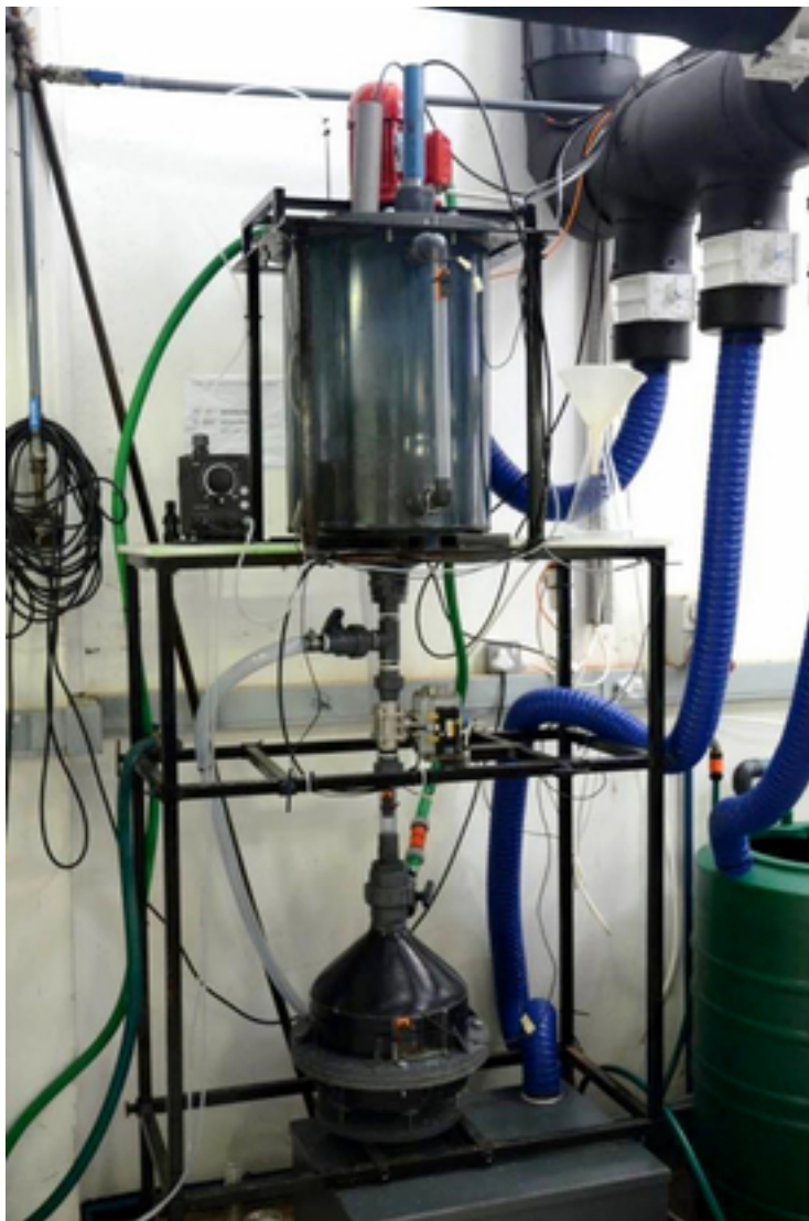
Automated separation of the mineral struvite from urine in a collaboration of Eawag with the University of KwaZuluNatal in South Africa. Struvite can be used as phosphorus fertiliser. (Photo: Eawag)
