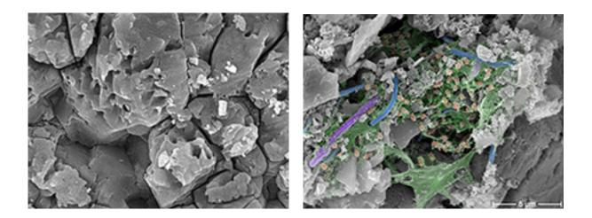
Scanning electron micrograph of limestone at t0 (left) and after a year in karst water (right). Staining was used to enhance the visibility of the biofilm, which includes bacterial cells (orange) and the associated polymer matrix (green). (*Photo: Inés Wilhartitz*)
