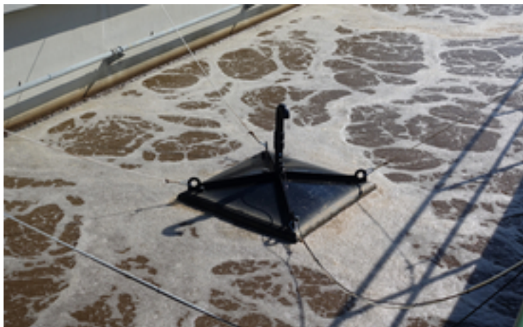
Off-gas measurement hood in operation at the Birs WTP. (Photo: Andrin Moosmann)
