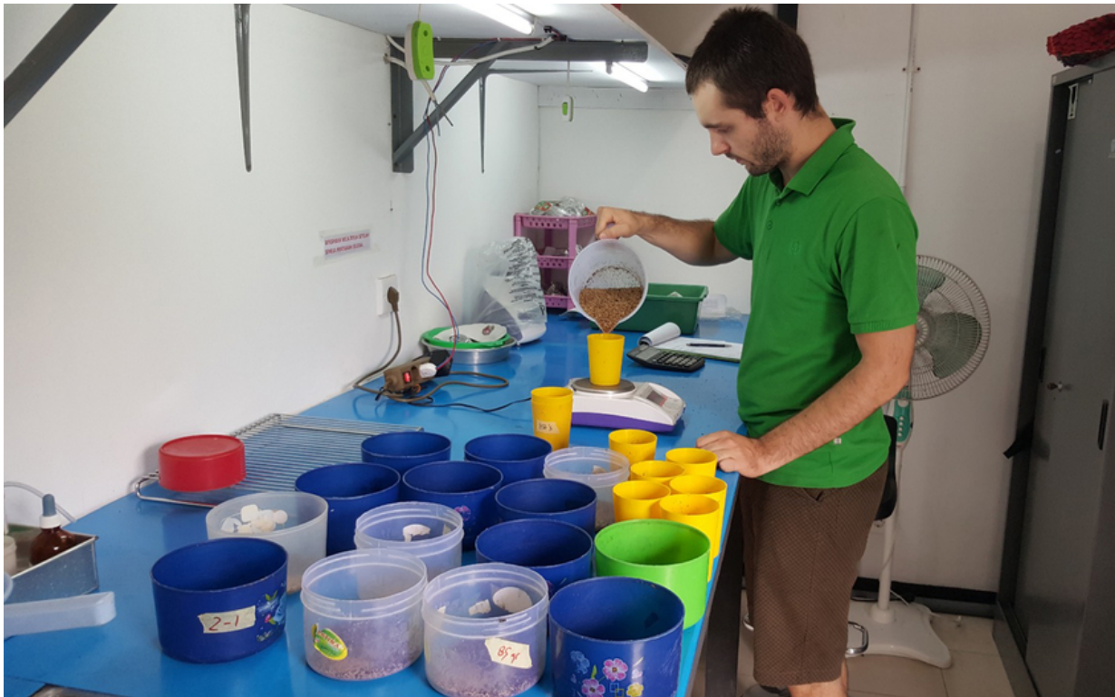
Bram Dortmans portions five-day-old fly larvae before adding them to organic waste (© Eawag).
