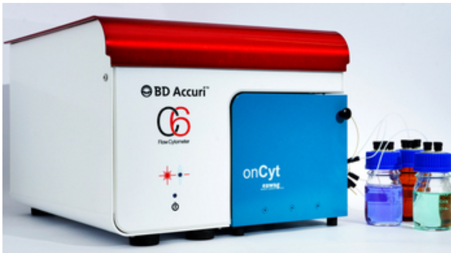
Fig. 2: Fully automated online flow cytometry system containing a conventional flow cytometer (red-white) and the automation module developed by Eawag (blue). Photo: Jürg Sigrist
