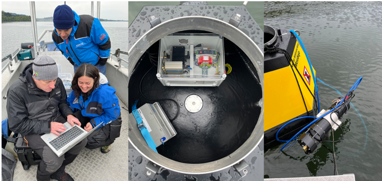
Left: Paul Roberts from the Monterey Bay Aquarium Research Institution calibrates the devices. Middle: View inside the buoy. On the right: The Aquascope underwater camera (Photos: Eawag).
