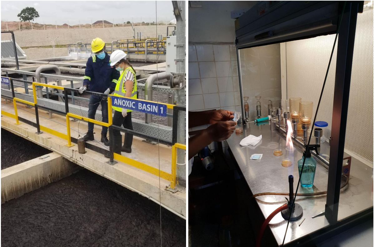
Figure 18: Photo of sampling procedure (left) and coliform analysis preparation (right)
