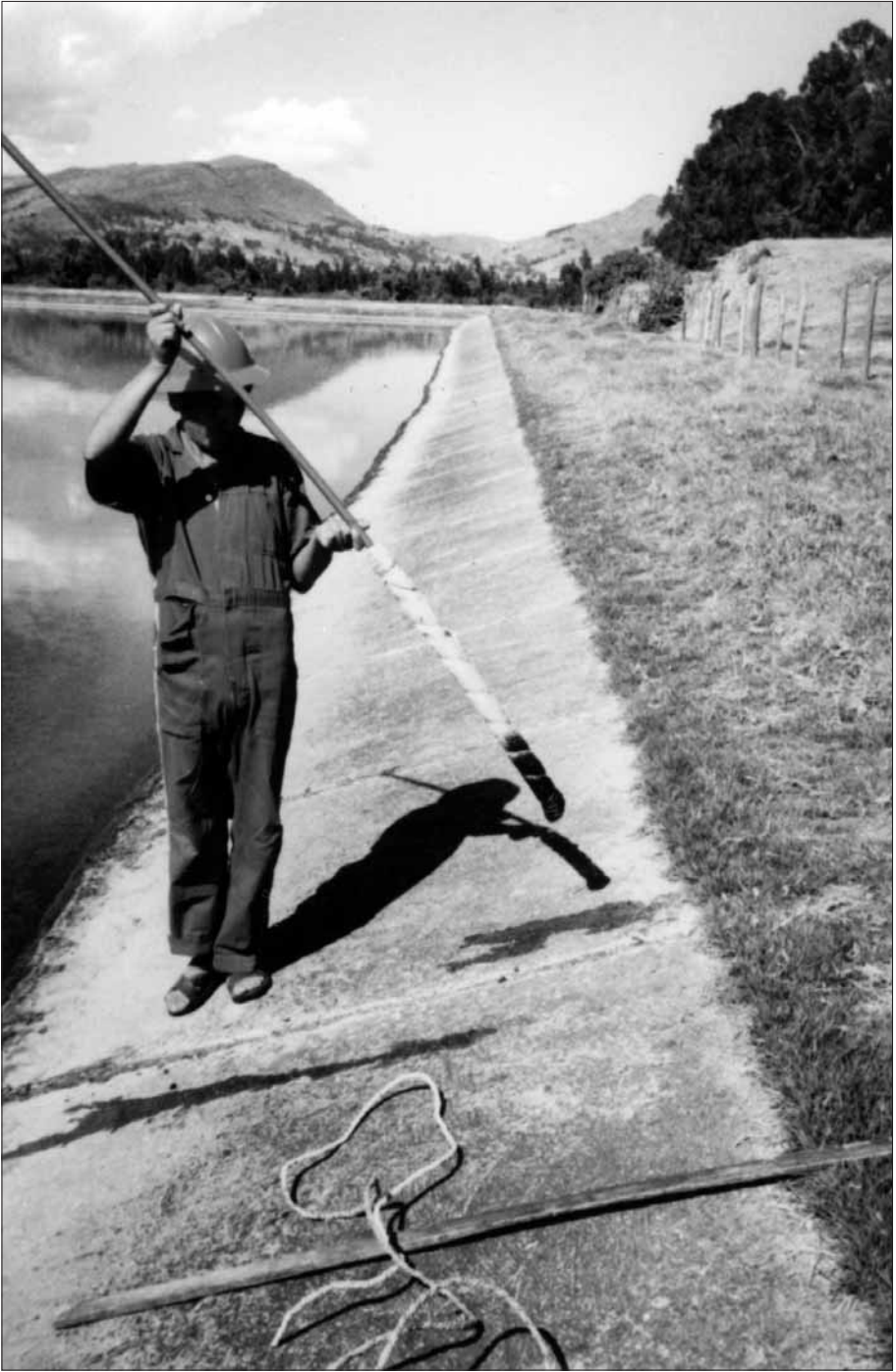
Figure 14.1 Sludge Depth Measurement by the 'White Towel' Test
