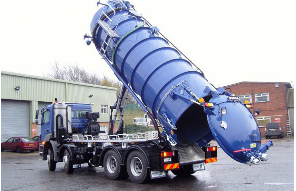
Figure 12. Emptying tanker by tipping (source: Vallely Vacuum Tankers, UK)
