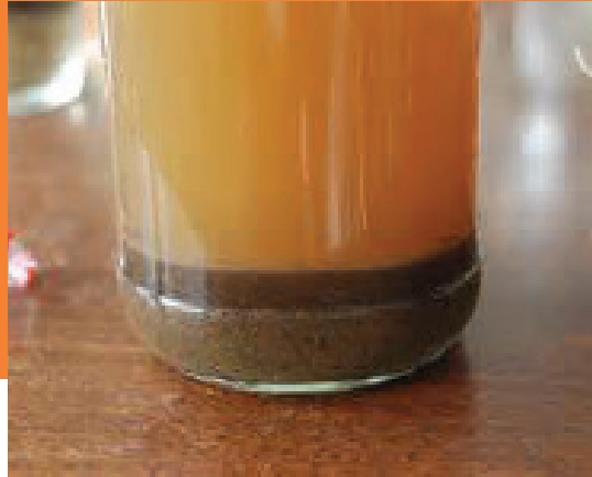
Figure 13. See the sample on the right? It is about 30% silt over 70% sand. The sand should be rejected and washed.
