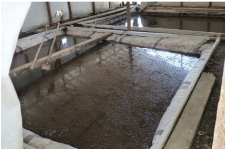
Figure 8. Lime stabilization reactor tank in Tacloban City, Philippines. It is an earthen pit lined with plastic and mixing is done manually.
