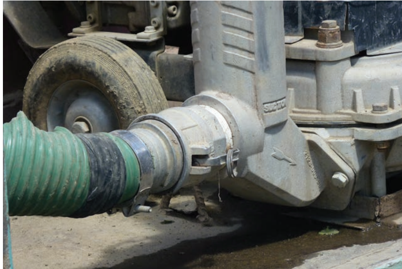
Figure 20. Quick couplers make for water tight fittings and allow rapid connections.
