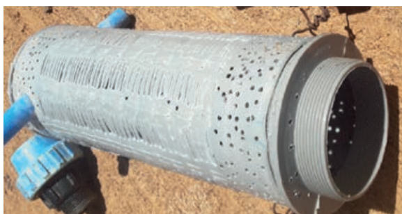
Figure 13: Perforated PVC pipe to protect strainer
