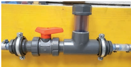
Figure 62: T-chlorinator in the laboratory at Eawag
