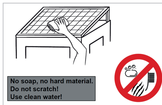
Figure 23: Instructions for cleaning the solar panel
