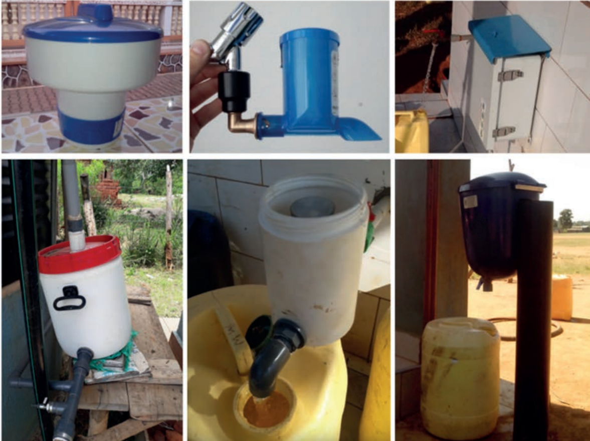
Figure 50: Alternatives to a T-chlorinator. From top left to bottom right: Floater, AquatabsFlo®, Venturi doser, Chlorine dosing bucket (CDB), Akvotur, Chlorine dispenser
