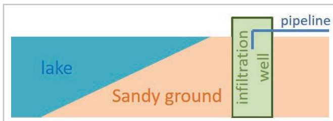
Figure 16: Scheme of an infiltration well
