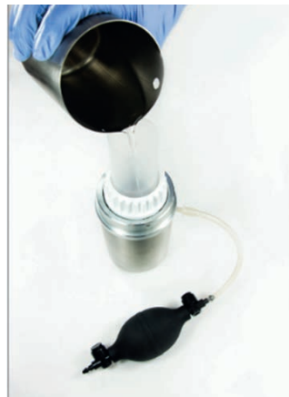
Figure 56: Membrane filtration funnel, DelAgua
