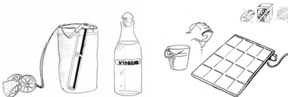
Clean Mini-WATA in a solution of water and lemon or vinegar
