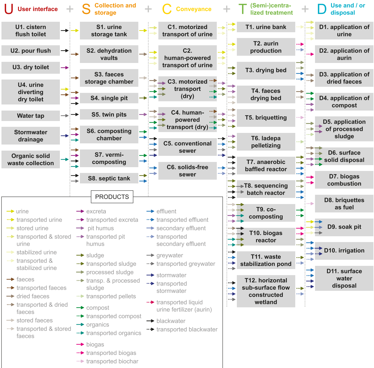
Fig. 2. Overview of the 41 technologies in this study used to generate sanitation systems and to quantify their substance flows grouped by functional group. Each technology is defined by its name, possible input and output products, and how these products relate to each other (e.g. 'OR' for either one or another, 'AND' if they always arise jointly). Taken from Spuhler et al. (2020b).
