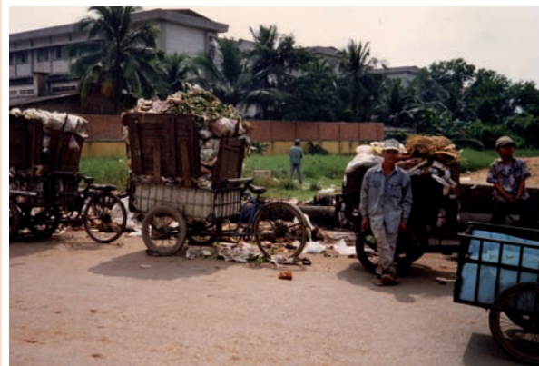
a) load in front of operator blocks view
