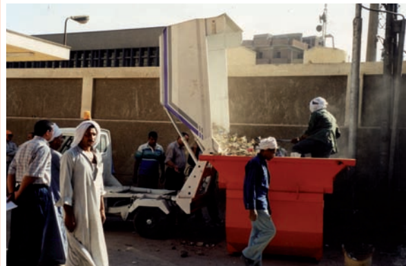
b) discharging load directly into container
