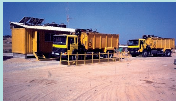
Photo 9.1 Weighbridge for collecting operational data
