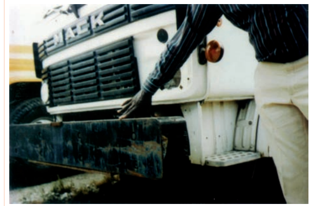
This truck was fitted with a small body because of the high waste density in Colombia. It then required a 1 ton ballast weight at the front to prevent it falling over backwards when unloading, thus further reducing its load capacity.
