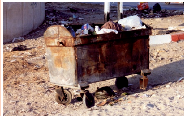
a) This wheeled container is difficult to move on uneven or soft ground, especially when the wheels are damaged because the containers are overloaded by dense waste
