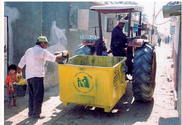
Photo 7.24 Loading container behind tractor
