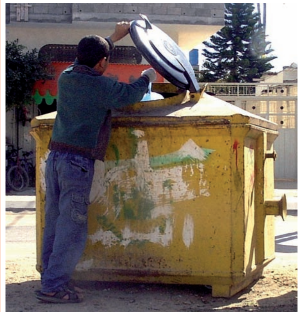
b) This container has no wheels and is picked up by a crane that can reach containers on the road verge (See Section 7.6.6)
