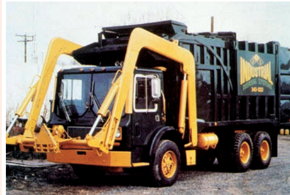
A costly system requiring a large area for manoeuvring. For low-density wastes.
