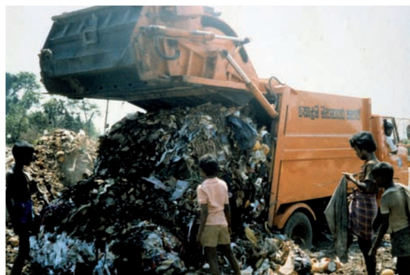
b) The waste is pushed out hydraulically by the compression (or ejector) plate
