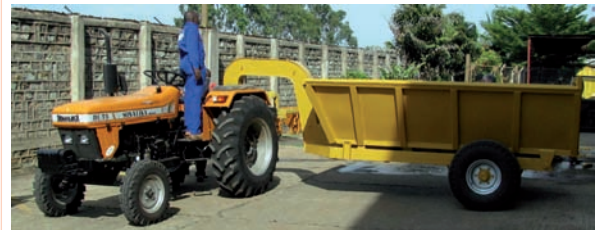
a) This design allows greater capacity and easier loading, and swan neck drawbar allows greater manoeuvrability
