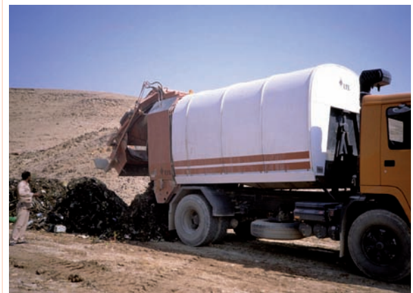
Photo 7.21 Rotating drum truck unloading
