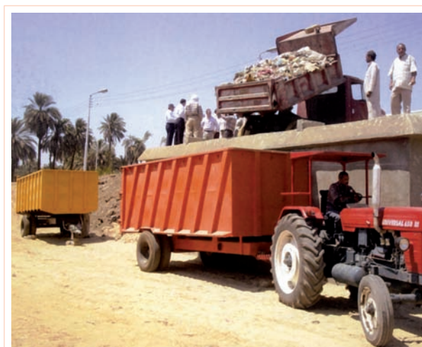
Note size of trailers, presence of spare trailer, and overhang to ensure waste does not fall between wall and trailer. For short-haul distances (up to 20 km) tractors with these large trailers are more efficient than trucks.
