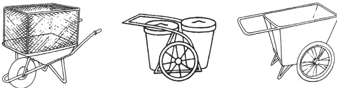
Figure 6.4 There many different types of street sweepers' handcarts which can be fabricated locally. (Each of these designs has drawbacks as well as advantages)
