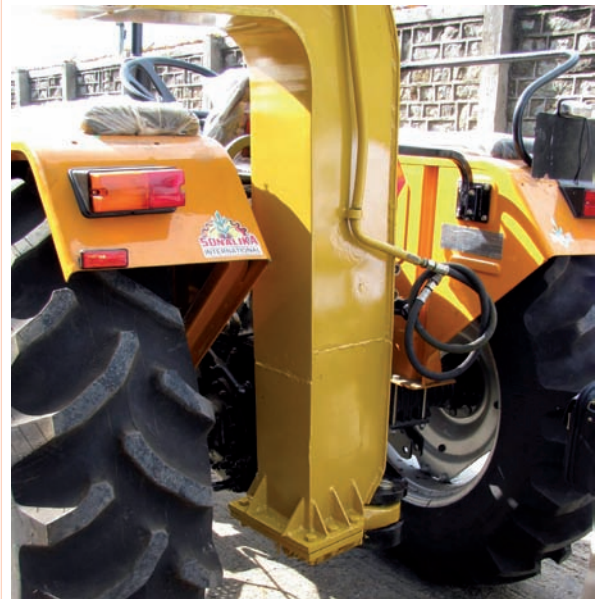
c) There must be sufficient clearance between the drawbar and the tractor wheels to allow for uneven ground
