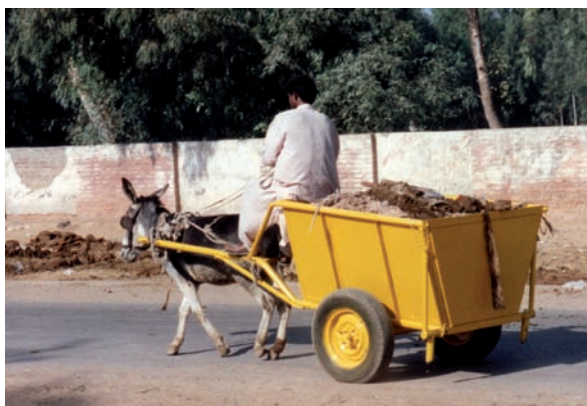
b) Redesigned cart & harness allows bigger payload, better weight distribution and easier tipping.
