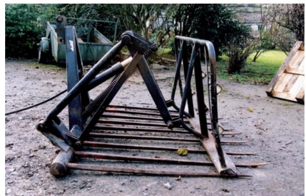
Photo A5.1 The agricultural buckrake for spreading wastes
