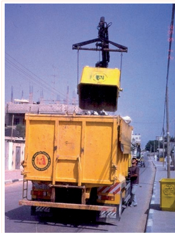
Photo 7.15 Crane tipper truck loading waste
