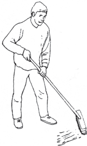
Stock broom – uses only the arm muscles, and covers a small area with each stroke
