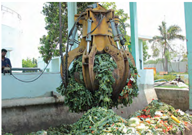
Collection of vegetable waste by a mechanical grab
