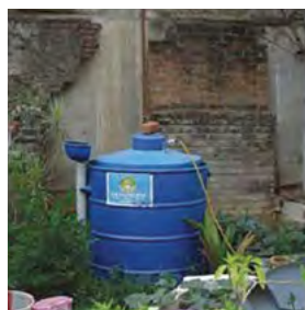
Biogas plants for processing organic waste; L- Model biogas plant for managing kitchen waste R-Temple Green initiative
