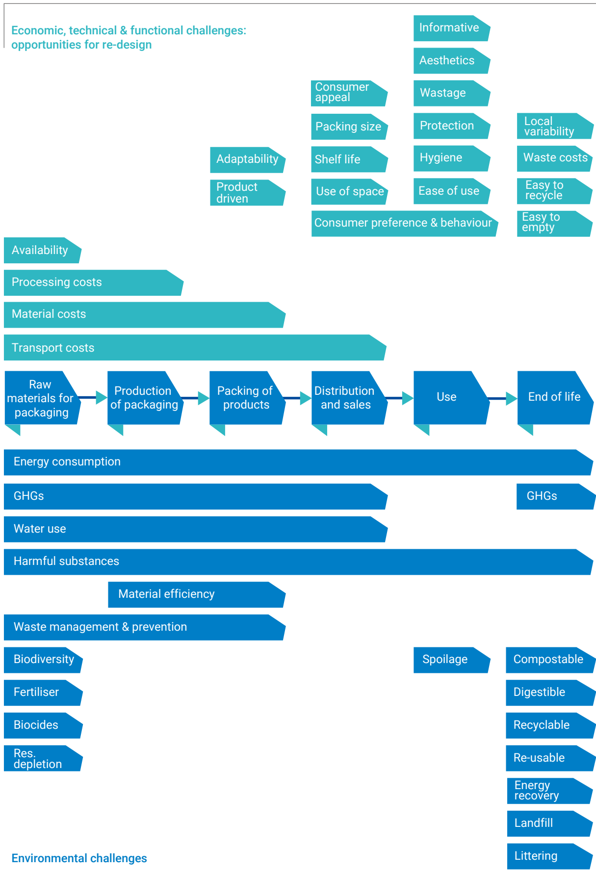
Figure 7.3 Environmental, economic, technical and functional challenges of the packaging value chain, adapted and further developed from Gronman et al. 2013.
