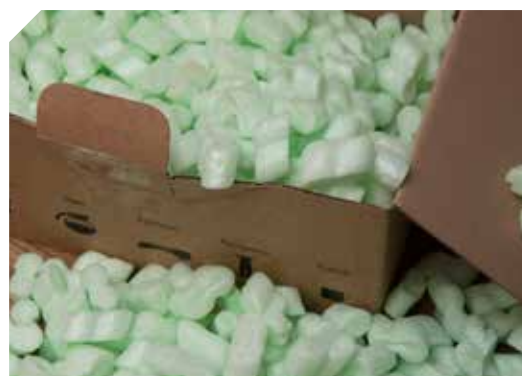
Figure 2.14 Loose fill used to protect goods in transit, made from EPS, ©Peter Kershaw.
