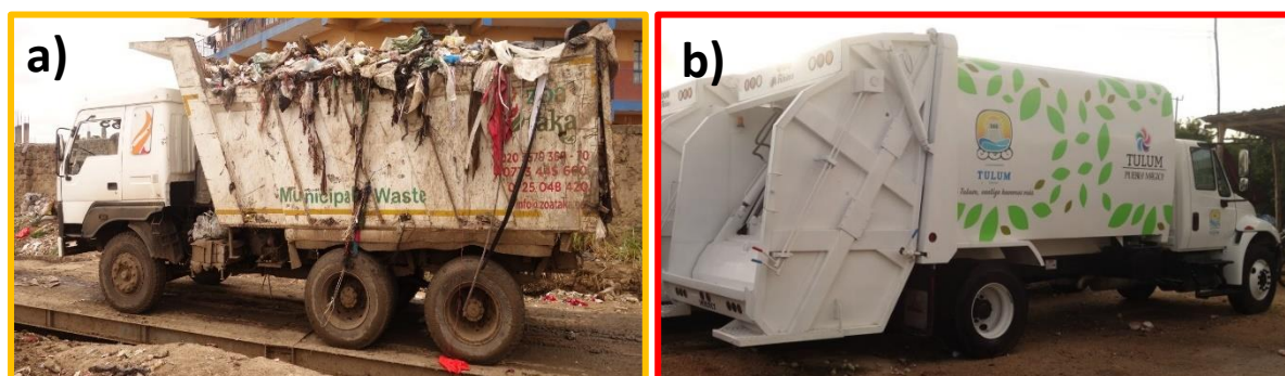
Figure 26: Collection vehicles carrying a) contained waste and b) uncontained waste
