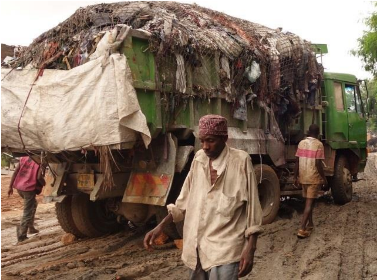
Figure 24: Load exceeds the capacity of the truck. Plastics leak from this secondary collection vehicle in Kenya.
