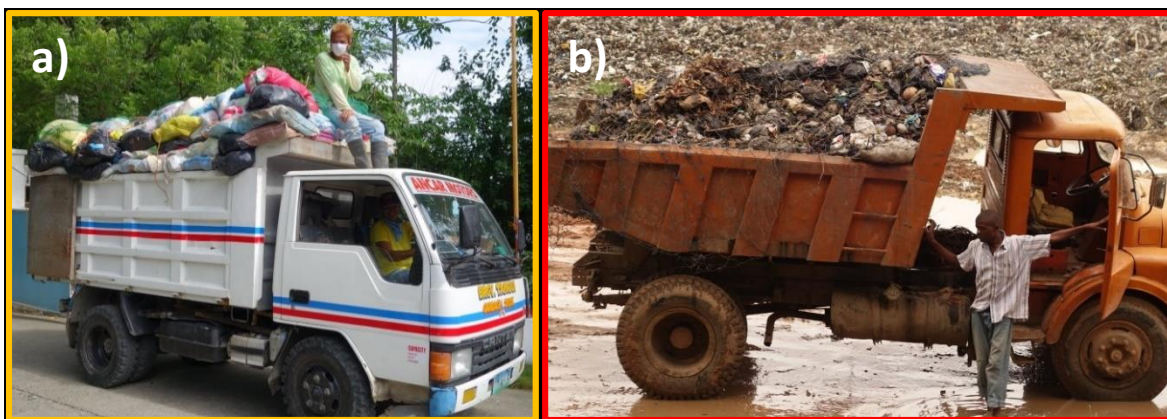
Figure 25: Collection vehicles carrying a) contained waste and b) uncontained waste
