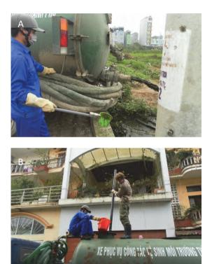
**Figure 3.19** A) collecting grab samples from the truck discharge valve to make a composite sample, and B) collecting a core sample from a truck access port with a 180 cm length PVC core sampling device with a 5 cm internal diameter, Hanoi, Vietnam (photos: Eawag).
