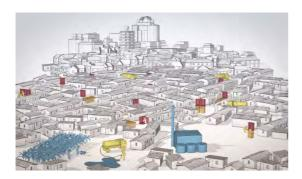
**Figure 1.1** An example of the role of integrated faecal sludge management in city-wide inclusive sanitation (CWIS), with networked solutions including sewer-based and non-sewer-based sanitation solutions. Colours illustrate the faecal sludge management service chain. Red: user interface; orange (underground): onsite containment; yellow: collection and transport; green: treatment; blue: end use as resource recovery (source: Eawag).
