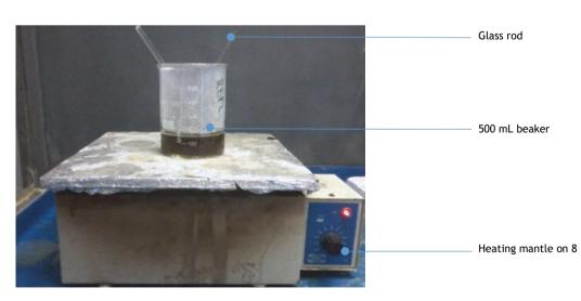
Figure 8.5 Acid-base digestion setup (photo: UKZN PRG).
