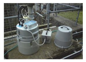
Figure 3.9 An automatic composite sampling device (photo: IHE Delft).
