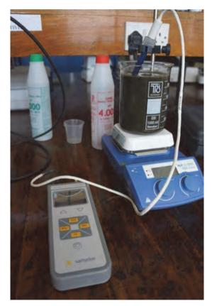
**Figure 8.10** Analysis of pH for liquid faecal sludge sample. Note position of pH electrode: submerged in the well-mixed sample, but with enough clearance above the magnetic stir bar (photo: Eawag).
