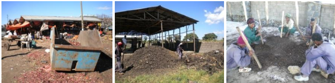
Figure 10: Municipal composting: Biowaste container in market, composting cite, crushing of compost (left to right)
