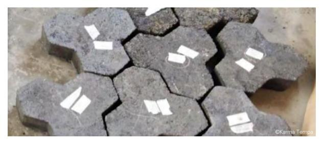
The process of making paving tiles is a downcycling method consisting of grinding plastic, melting it, mixing it with sand and eventually pouring it in tile molds before cooling.
