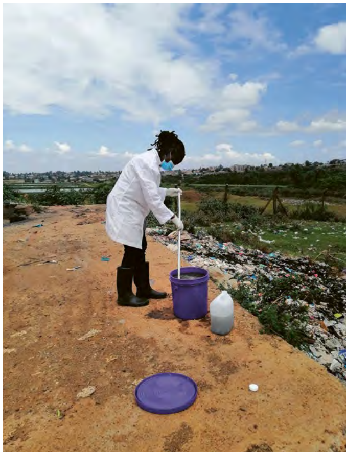
Photo 1: Ednah Kemboi collecting faecal sludge samples at the Quarry Wastewater Treatment Plant. The faecal sludge was analysed for dewatering performance and stabilisation level in the laboratory at Eawag.
