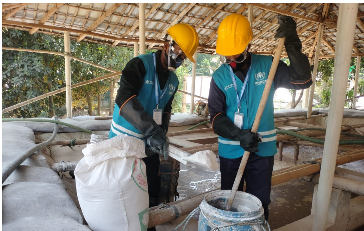
Figure 11: Two operators at the treatment plant in Cox's Bazar, Bangladesh, are making a lime slurry (source: UNHCR).
