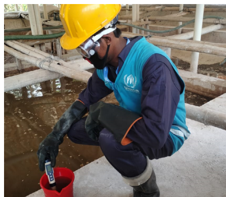
Figure 13: A staff member at the faecal sludge treatment plant in Cox's Bazar measures pH of the lime-treated sludge (source: UNHCR).
