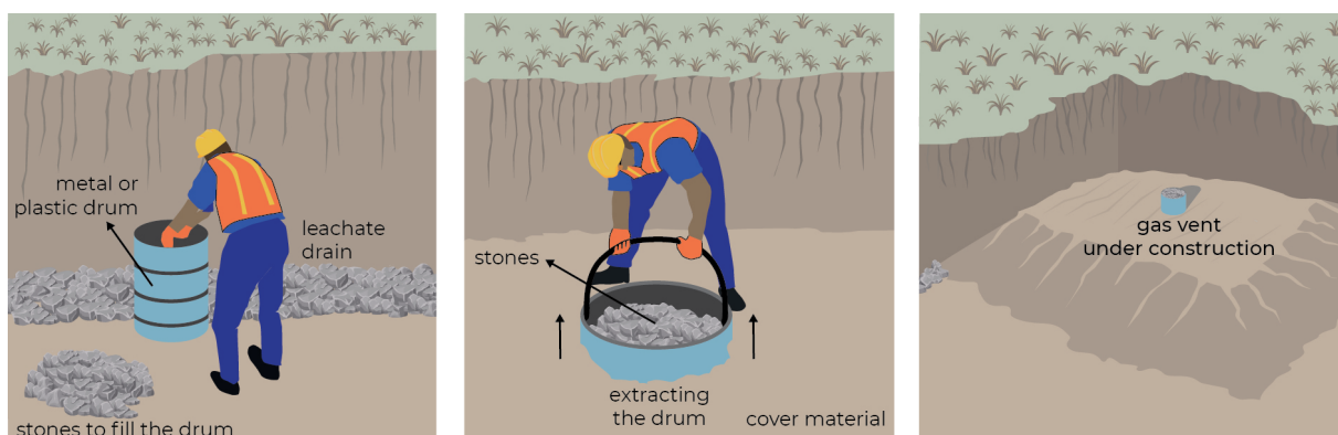
Figure 23: Gas vent construction
