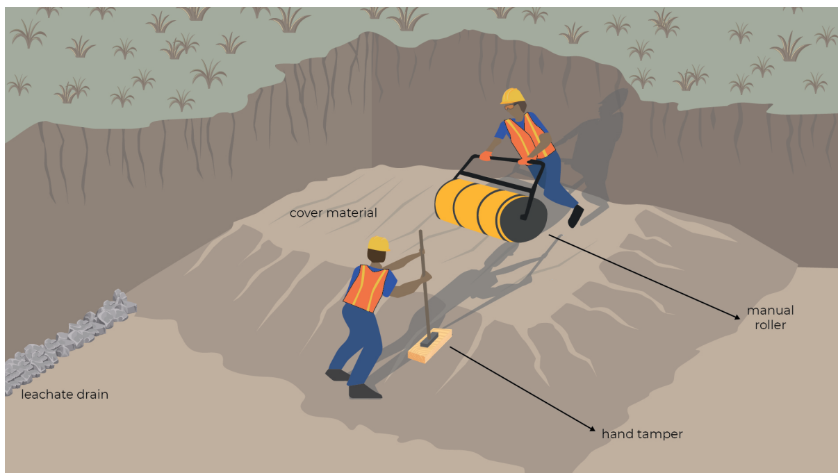
Figure 11: Final compaction and closure of the cell
