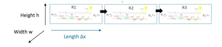
Assumption: In our model the boxes are completely mixed reactors. Therefore the longitudinal dispersion coefficient (eq. 6.65) is determined by the length of the boxes. If we choose a length that is too large, the mixing will be unrealistically large as well.
