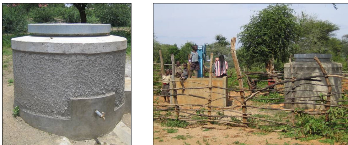
Figure 3-3: The picture on the left shows a remote community filter for treating surface water. The picture on the right shows a remote community filter that is attached to a hand pump unit for pumping groundwater.
