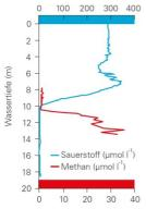
Typical profiles of oxygen and methane concentrations in Lake Cadagno. Methane consumption occurs in a relatively thin water layer at a depth of 10–13 metres. (Data: Eawag / MPI-Bremen)
